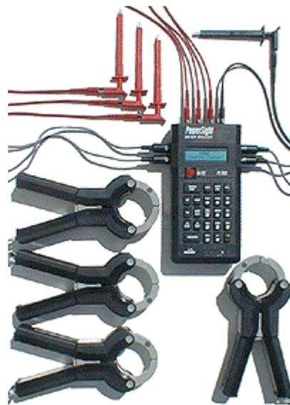
**Figure 2- Three Phase Power Meter**
