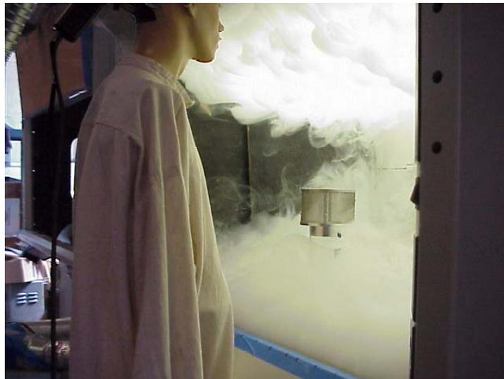
**Fig 8** – Run #1, 50 percent airflow, mannequin at 26 inches above work surface (note ejector).
