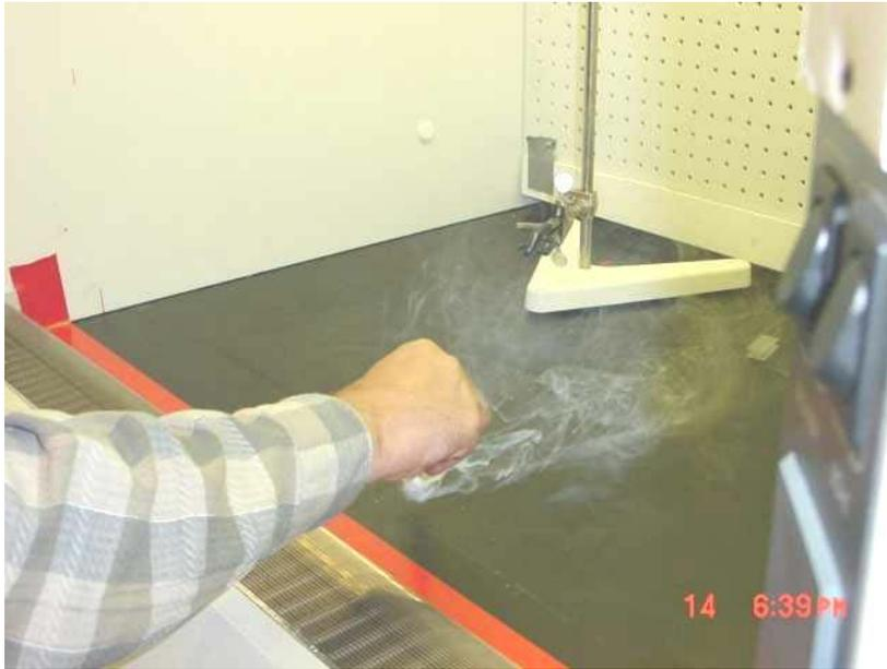
**Fig. 5** – SDSU Berkeley hood demonstrating floor sweep with point-source smoke.
