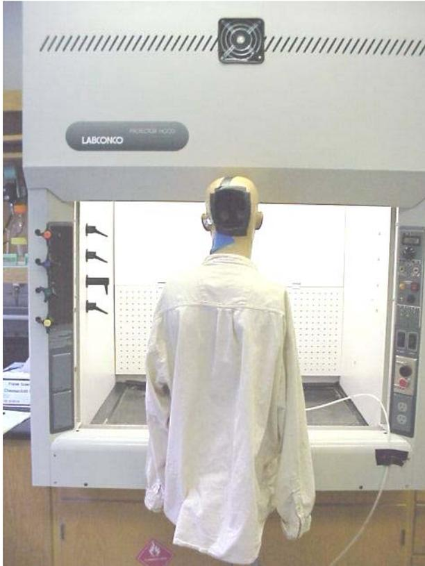
**Fig. 1** – Mannequin position for standard ASHRAE 110 SF6 test; 26 inches above, Center.
